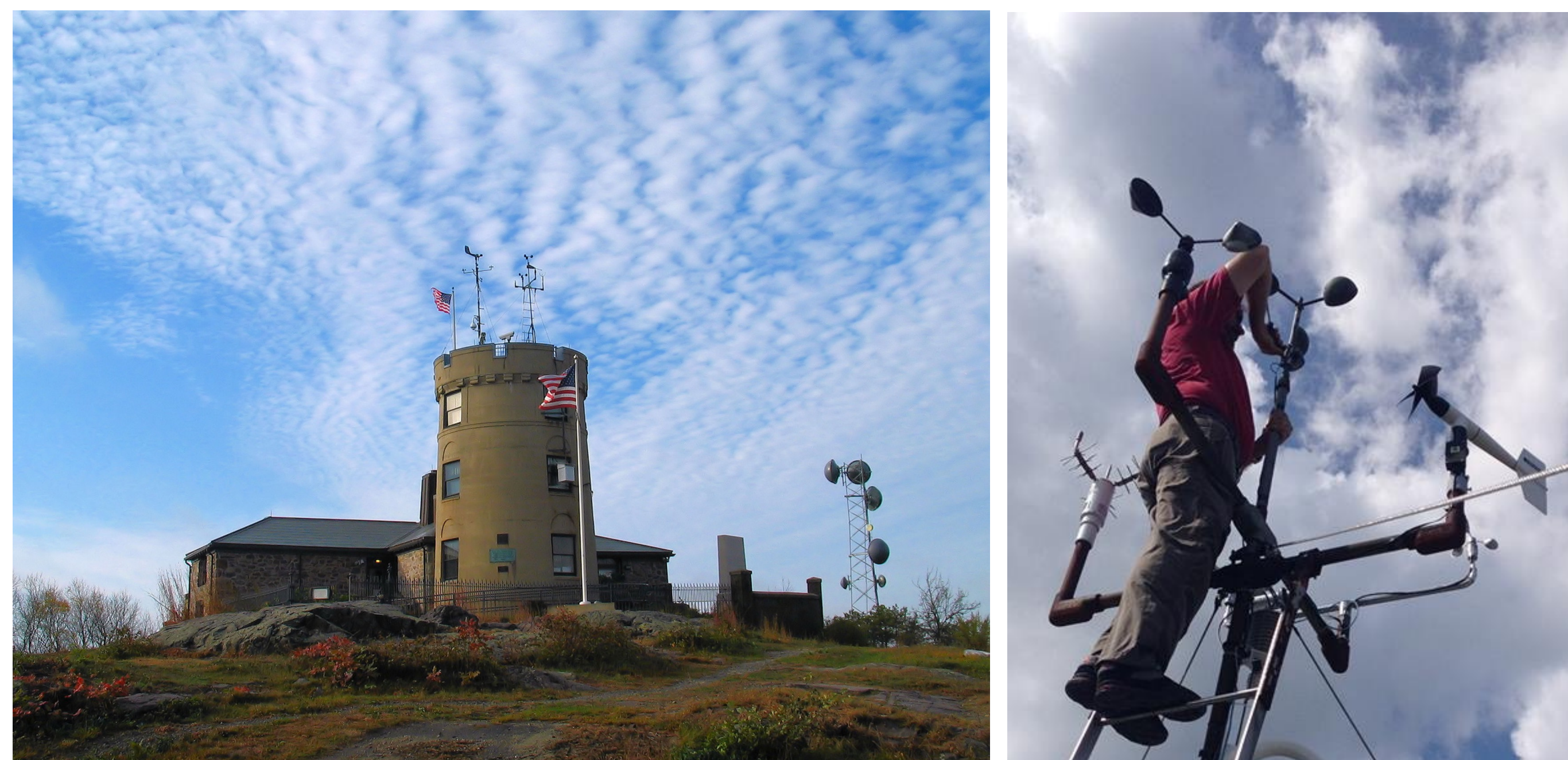
Blue Hill Observatory's Program Director Don McCasland on the wind tower adding oil to the 1960s-era contacting anemometer, allowing wind records to continue using historically similar recording devices to those once available in the 1880s.
